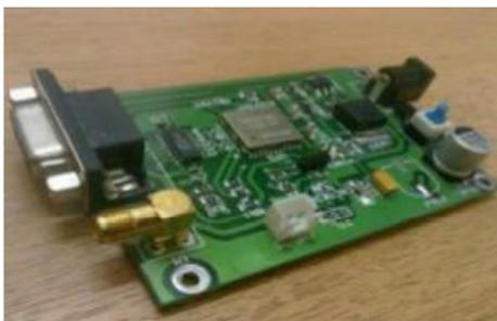
The GSM modem can be used for communication like messages. To and from the owner. It is a typical type of modem in which contains SIM card, and operates over a subscription to a mobile operator, just like a mobile phone. From the mobile operator view
