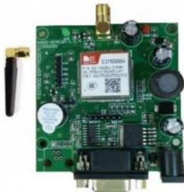
GSM means Global system module is used for communication. A sim card has to be inserted for communication. Messages can be received for defined number using sim card. Time Division Multiple Access method is used for this process. It can communicate mobile, Computer over a network. It can also be connected to the computer through Bluetooth or serial ports. It has the abilities to make a call or send a message and it can delete messages also in the SIM card that are received or send by the GSM.
